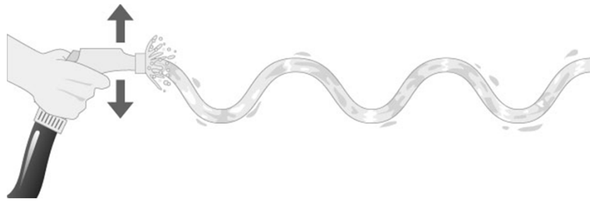
Figure 2-8 Simulating a radio wave using a garden hose
