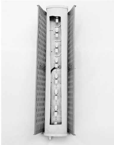
Figure 4-7 Cellular antenna with cutout to show internal construction
